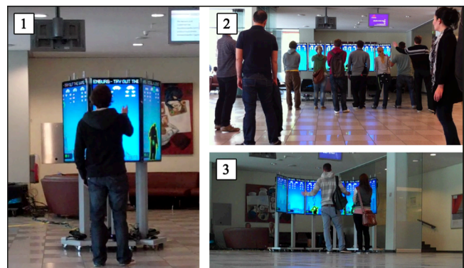
Figure 1: Chained Displays : (1) Hexagonal : actors can limitedly see other screens resulting in low social learning (2) Flat attracts more people (Honeypot) because actions and their effects can be observed (3) Concave : actors have a limited interaction space resulting in few simultaneously interacting users.
